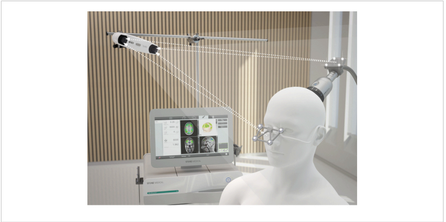
Figure 2: MRI navigation system. The image illustrates the ideal alignment between the patient and the NEUROLITH during TPS. The 3D camera contacts the detection lenses of the goggle and those of the handpiece. Only if this transmission is guaranteed is the handpiece recognized in the correct spatial position and the visualization of the stimulation on the screen is undisturbed. This figure has been modified from 9 . Please click here to view a larger version of this figure.
